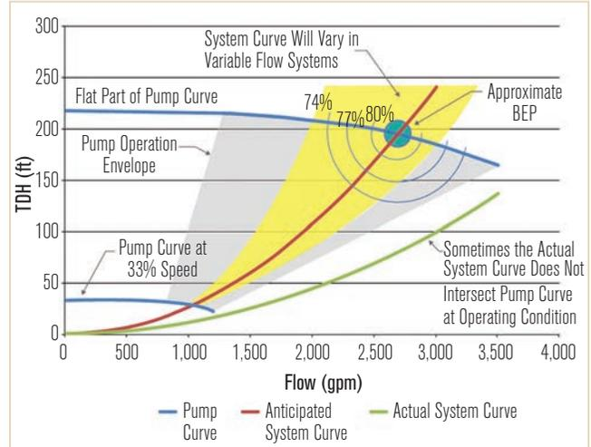
FIGURE 2 Pump and system curves.
