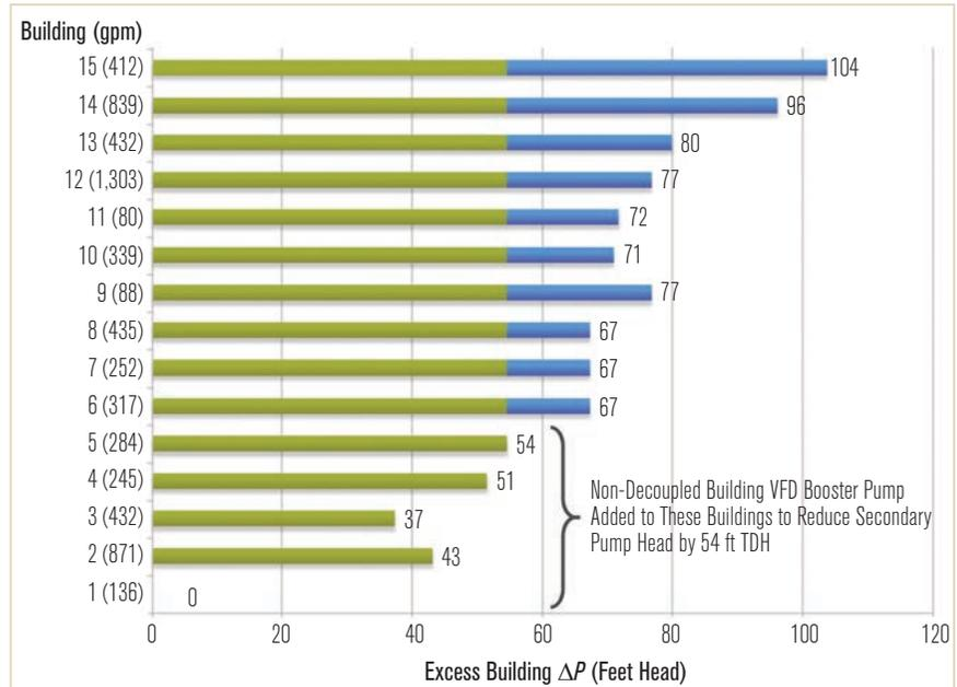
FIGURE 1 Example of multibuilding CHW system  $\Delta P$  requirement valuation.
